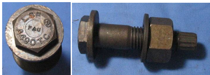
Figure 5-11 A490 Bolts in Slip Load Tests
