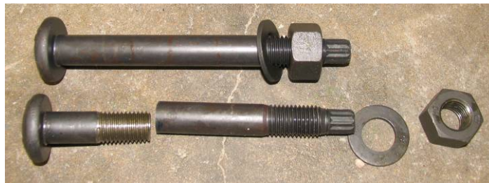
Figure 3-20 7 inches long A490 bolt was shortened for block shear tests
