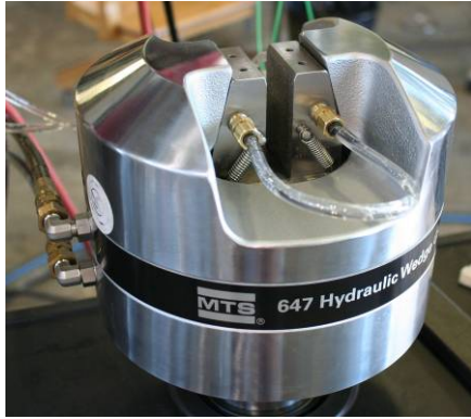
Figure 3-28 Water Cooled Wedge
