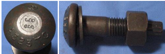
Figure 3-18 A325 bolt in single bolt connection test
