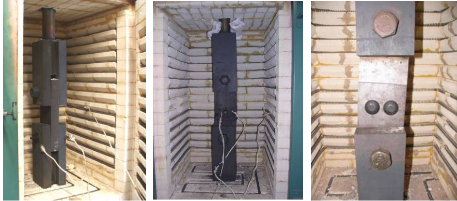
(a) Bolt Shear Test (b) Single Bolt Connection (c) Two Bolt Connection
