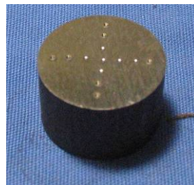
Figure 5-3 Layout of Hardness Test Points on Bolt Section and Tested Bolt Segment
