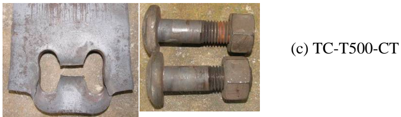
Figure 6-15 Block Shear Failures at Different Temperature Levels (Constant Temperature Tests) (Continued)
