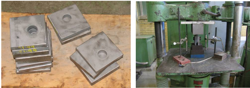
Figure 3-23 Steel Plates after Sand Blasted Figure 3-24 Slip load Test
