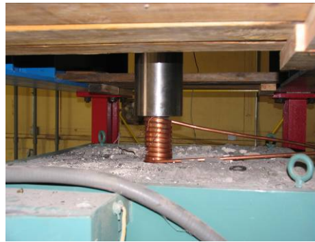
Figure 3-10 Water Cooling System
