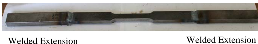
Figure 7-11 Coupon of 3/8 inch Gr. 50 Steel with Welded Extension
